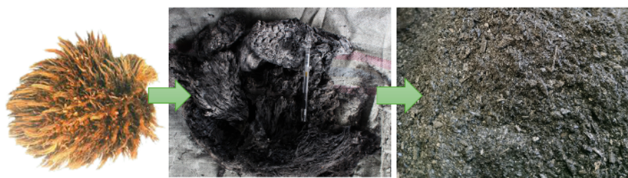
Fig. 2. EFB biochar produce from conventional brick dome kiln.
