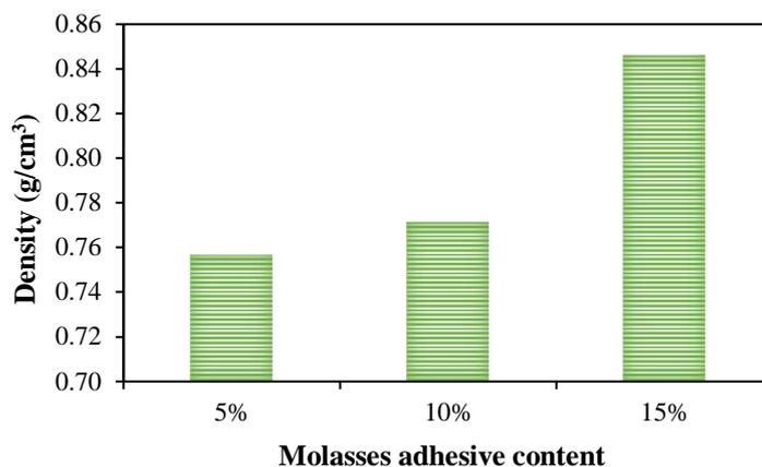
**Fig. 3.** The density value of sawdust bio-charcoal briquettes at various adhesive concentrations.
