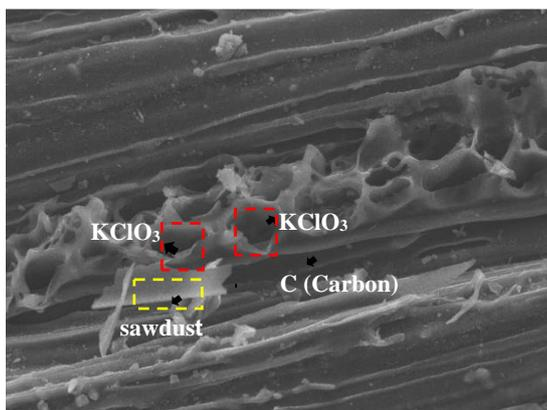
**Fig. 5.** SEM results on sawdust bio-charcoal briquettes.
