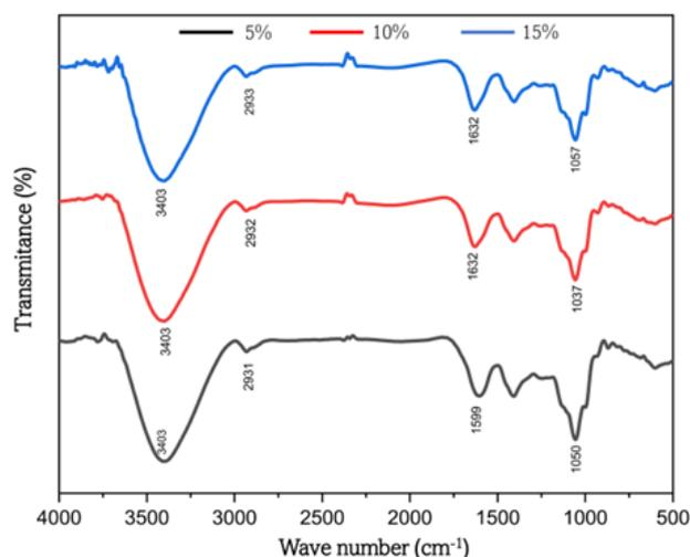
**Fig. 7.** FTIR spectra of sawdust bio-charcoal briquettes at varying concentrations of molasses adhesive.
