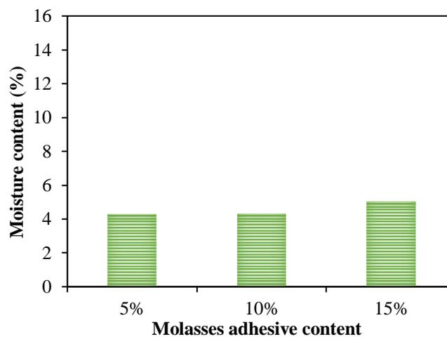
**Fig. 4.** The moisture content of sawdust bio-charcoal briquettes at various adhesive concentrations.
