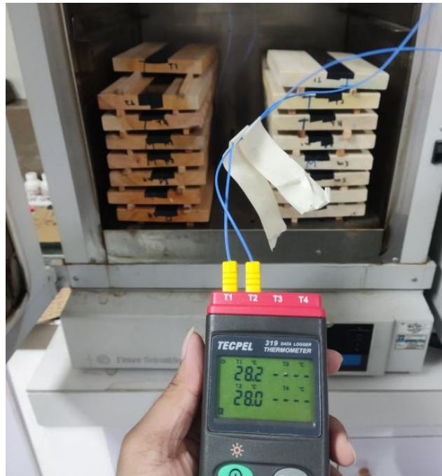
Fig. 1. Setup for heating wood samples using a Fisher Scientific Isotemp 650G oven.
