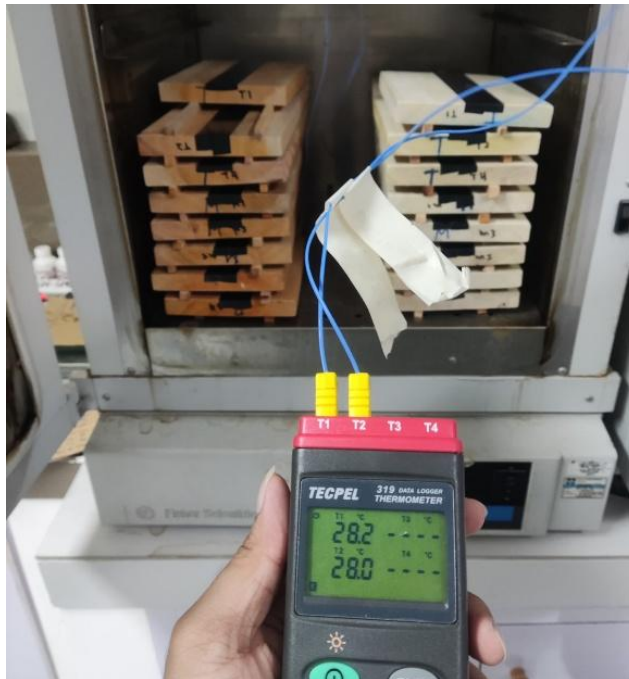
Fig. 1. Setup for heating wood samples using a Fisher Scientific Isotemp 650G oven.
