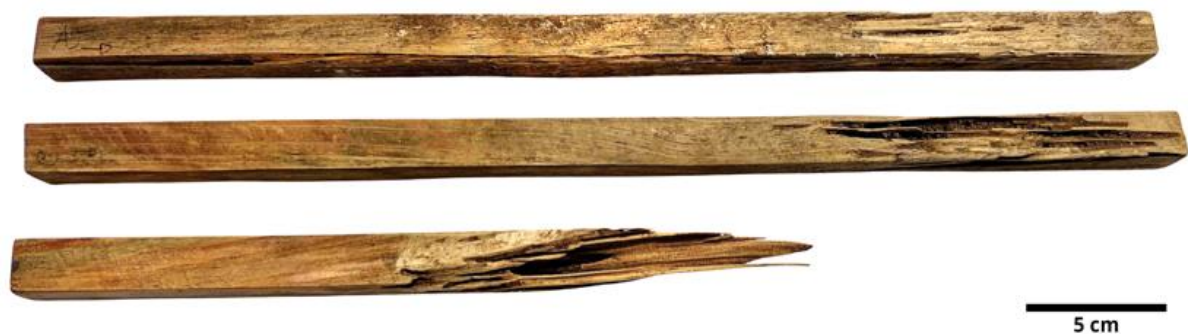
Fig. 7. Damage to wooden baits caused by termites: (a) Nasutitermes sp. in Dufa-Dufa Village, North Ternate Sub-district, (b) Microcerotermes sp. in Gambesi Village, South Ternate Sub-district, (c) Coptotermes sp. in Malikrubu Village, Central Ternate Sub-district.
