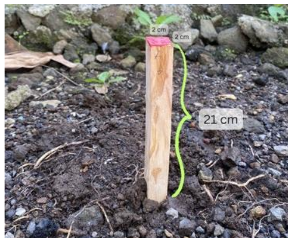
Fig. 2. Termite bait wood installation.
