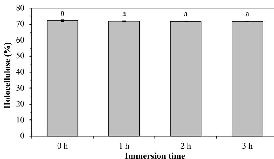
**Fig. 1.** Holocellulose content of betung bamboo due to alkali immersion treatment at various immersion times (Different letters show significant differences between treatments according to Duncan's multiple range tests at a 5% confidence interval. Error bars show standard deviation).
