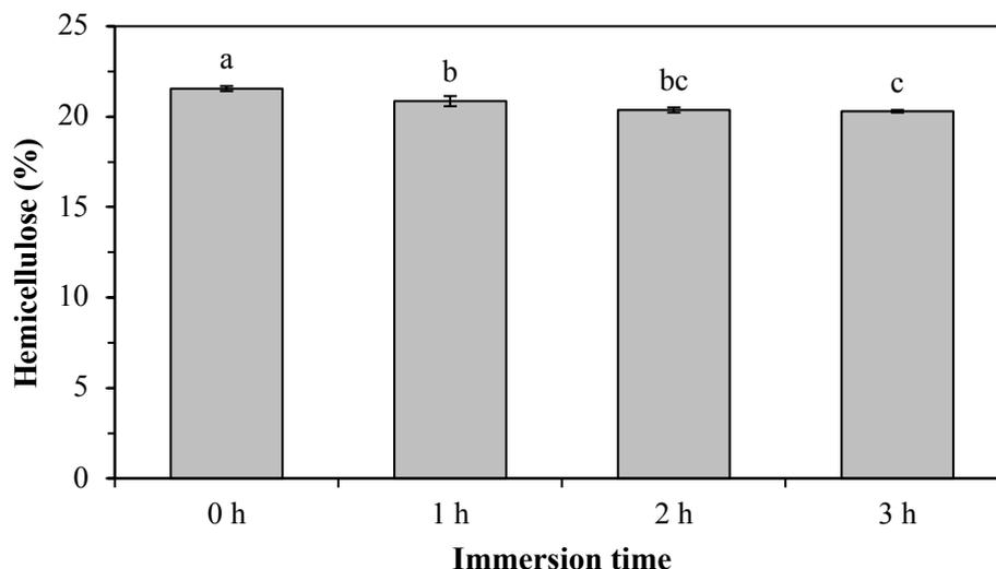
**Fig. 3.** Hemicellulose content of betung bamboo due to alkali immersion treatment at various immersion times (Different letters show significant differences between treatments according to Duncan's multiple range tests at a 5% confidence interval. Error bars show standard deviation).
