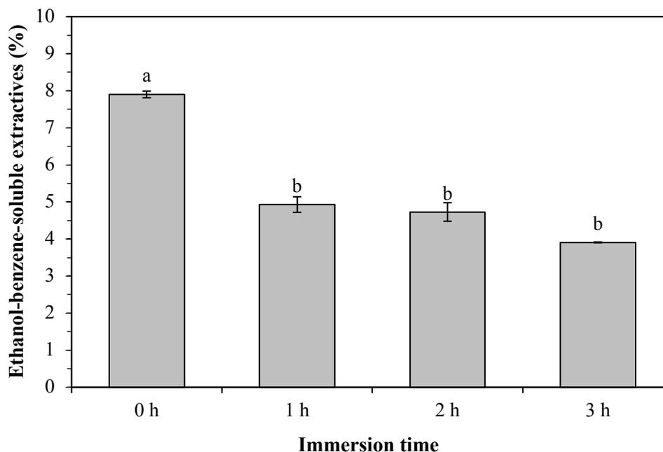
**Fig. 8.** Ethanol-benzene-soluble extractives content of betung bamboo due to alkali immersion treatment at various immersion times (Different letters show significant differences between treatments according to Duncan's multiple range tests at a 5% confidence interval. Error bars show standard deviation).
