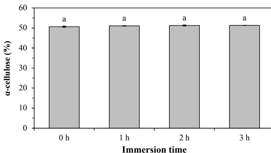
**Fig. 2.**  $\alpha$ -cellulose content of betung bamboo due to alkali immersion treatment at various immersion times (Different letters show significant differences between treatments according to Duncan's multiple range tests at a 5% confidence interval. Error bars show standard deviation).
