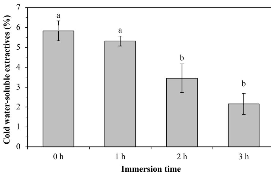
**Fig. 5.** Cold water-soluble extractives content of betung bamboo due to alkali immersion treatment at various immersion times (Different letters show significant differences between treatments according to Duncan's multiple range tests at a 5% confidence interval. Error bars show standard deviation).
