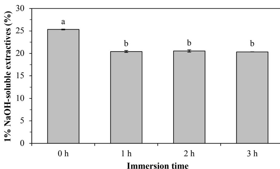
**Fig. 7.** 1% NaOH-soluble extractives content of betung bamboo due to alkali immersion treatment at various immersion times (Different letters show significant differences between treatments according to Duncan's multiple range tests at a 5% confidence interval. Error bars show standard deviation).
