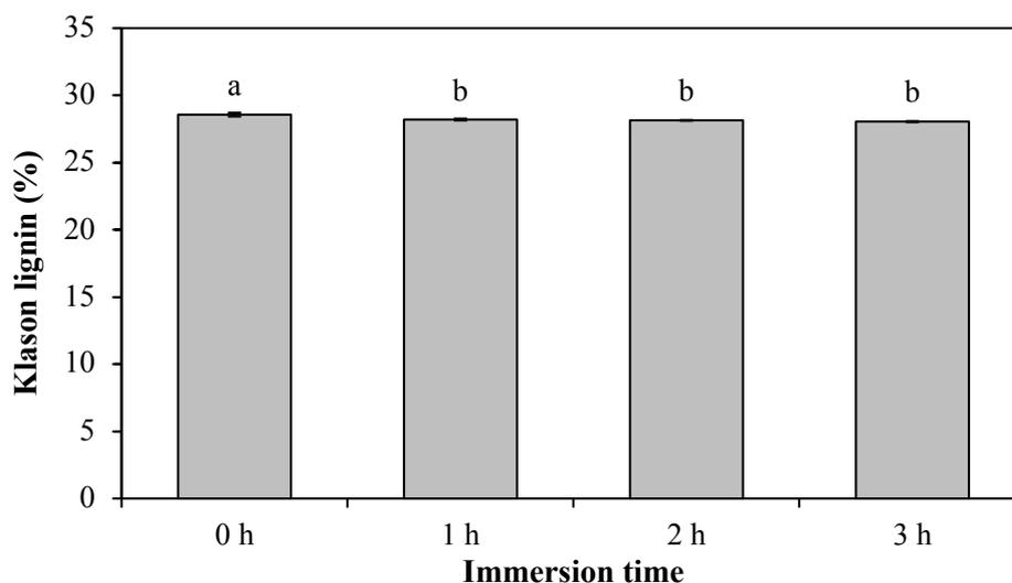
**Fig. 4.** The lignin content of betung bamboo due to alkali immersion treatment at various immersion times (Different letters show significant differences between treatments according to Duncan's multiple range tests at a 5% confidence interval. Error bars show standard deviation).
