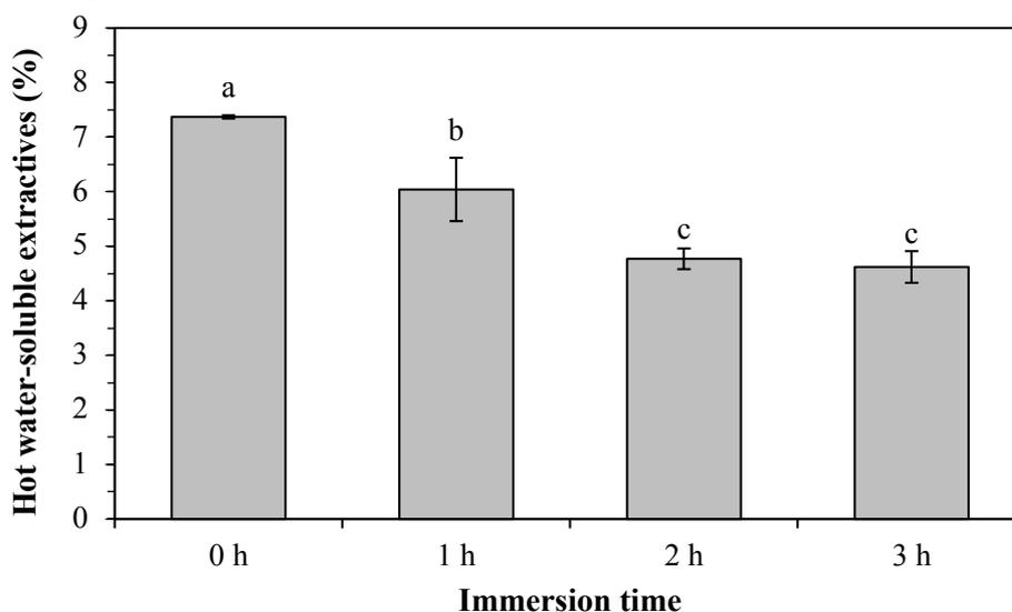
**Fig. 6.** Hot water-soluble extractives content of betung bamboo due to alkali immersion treatment at various immersion times (Different letters show significant differences between treatments according to Duncan's multiple range tests at a 5% confidence interval. Error bars show standard deviation).
