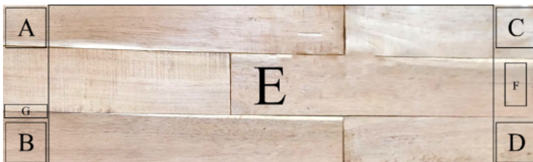
Fig. 1. Test sample cutting pattern. (A= test sample of density, moisture content, and volume shrinkage ( 3.6 \times 7.5 \times 7.5 ) cm 3 , B = test sample of water delamination, WA, and TS ( 3.6 \times 7.5 \times 7.5 ) cm 3 , C= test sample of boiling delamination ( 3.6 \times 7.5 \times 7.5 ) cm 3 , D= test sample backup ( 3.6 \times 7.5 \times 7.5 ) cm 3 , E= test sample of MOE and MOR ( 3.6 \times 30.0 \times 85.0 ) cm 3 , F= test sample of block shear parallel to the grain ( 3.6 \times 2.0 \times 5.0 ) cm 3 , G= test sample of block shear perpendicular to the grain ( 3.6 \times 4.0 \times 5.0 ) cm 3 ).
